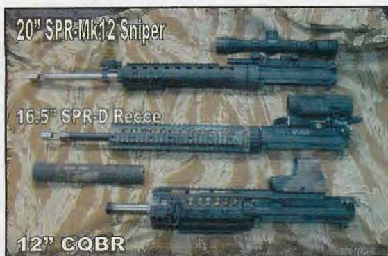
Three early experimental 6.8 upper-receiver groups show a conceptual SPR Mk-12, a 16.5-inch barrel SPR-D, and a 12-inch barrel CQB (Close-Quarter-Battle) version. The middle component is one of the first mid-length gas systems to be tested and was the basis for the “Recce” rifle. The CQB version was designed to function with the OPS, Inc. SOPMOD suppressor.
